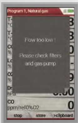
Optional gas flow monitoring (e. g. clogged filter)
