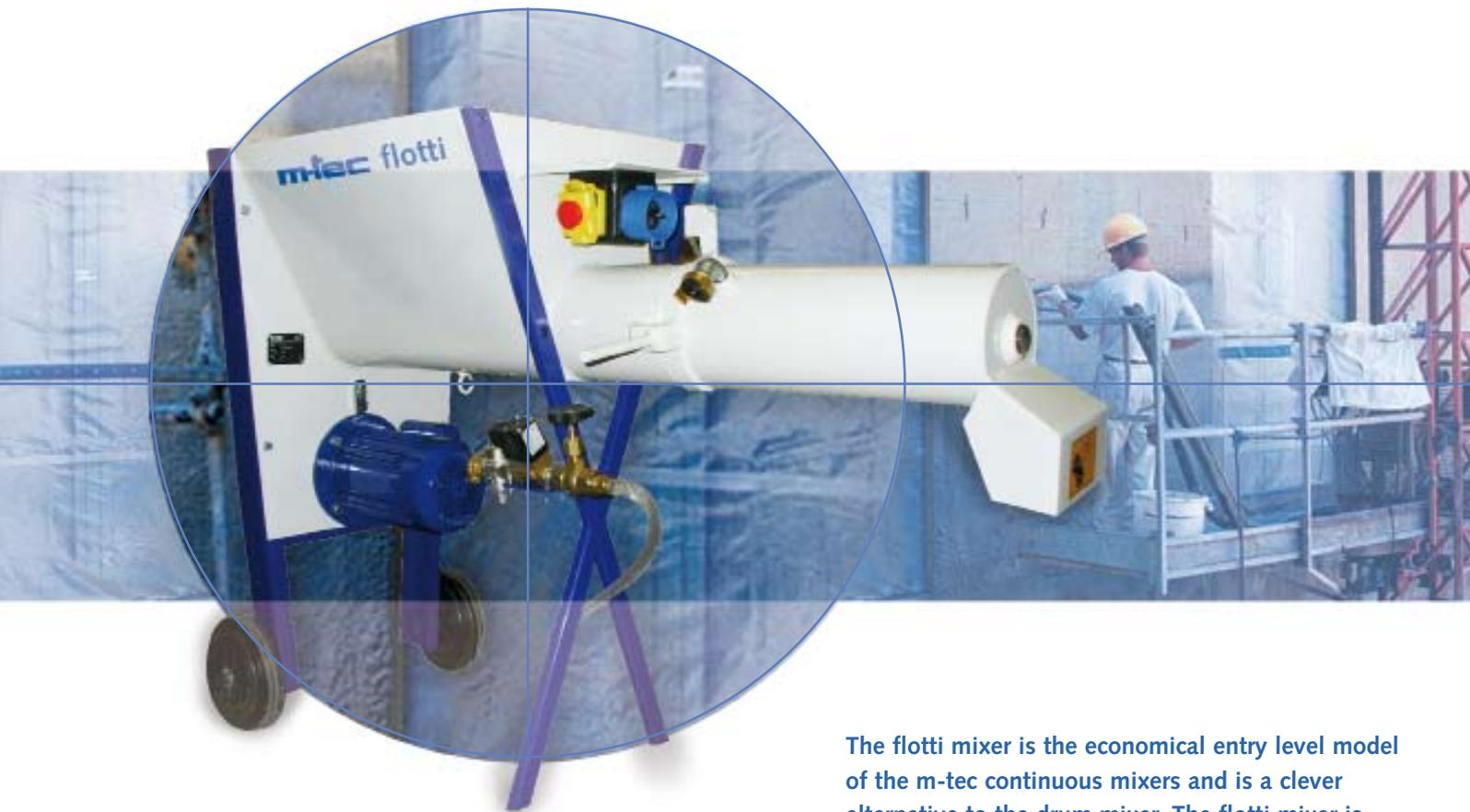
The flotti mixer is the economical entry level model of the m-tec continuous mixers and is a clever alternative to the drum mixer. The flotti mixer is used to process ready-mix dry mortars, such as bricklaying mortars, plaster and cement mortar, tile adhesive, anhydrite floor screed or decorative renders in a granularity of up to 4 mm.
